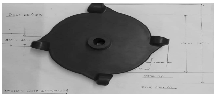
Fig.3 view of fertilizer metering cup feed plate
